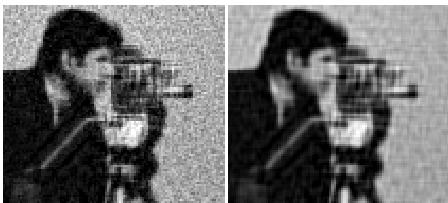
Fig. 3. Result of the pure regularized inverse z^{RI} from (8) (left) and the "oracle" Wiener estimate, ISNR=5.22 dB (right).
