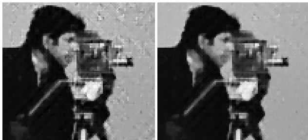
Fig. 5. Filtering the Poisson data with the algorithm developed for the Gaussian one. Standard selection of the algorithm parameters gives a poor estimate, ISNR=5.38 dB (left). Up to some extent, it can be improved by manually optimizing some algorithm parameters, ISNR=6.03 dB (right).
