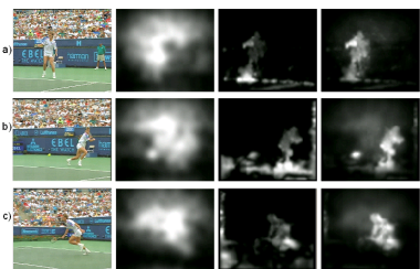
Fig. 3. Example of spatio-temporal saliency maps for the sequence Stefan . From the left to the right, we have spatial, temporal and spatio-temporal saliency map.
