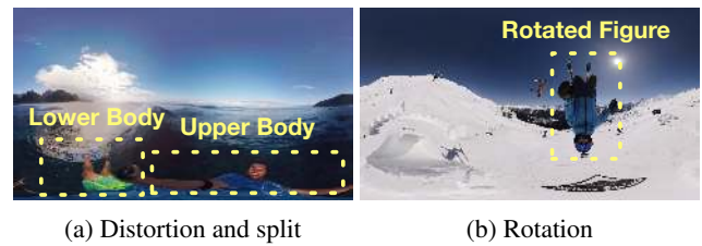
Figure 2: Distortion and rotation problems in 360 videos
