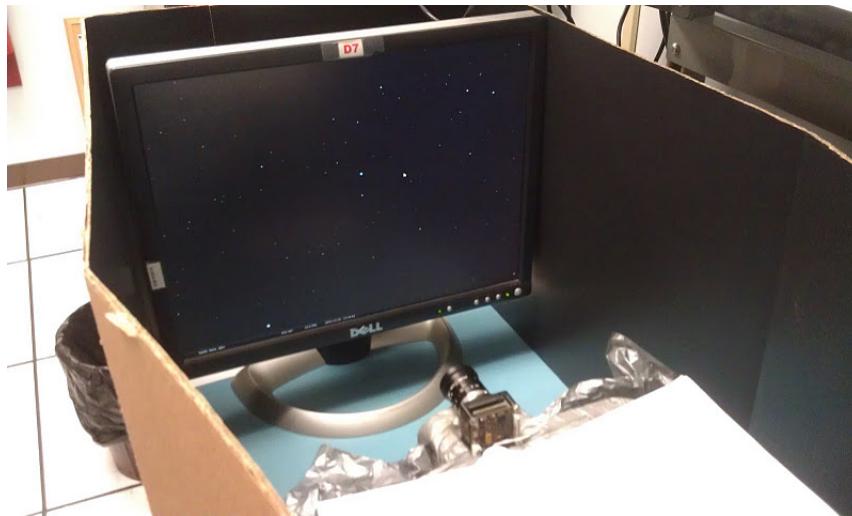
Figure 5.6: Simulated star field setup.
