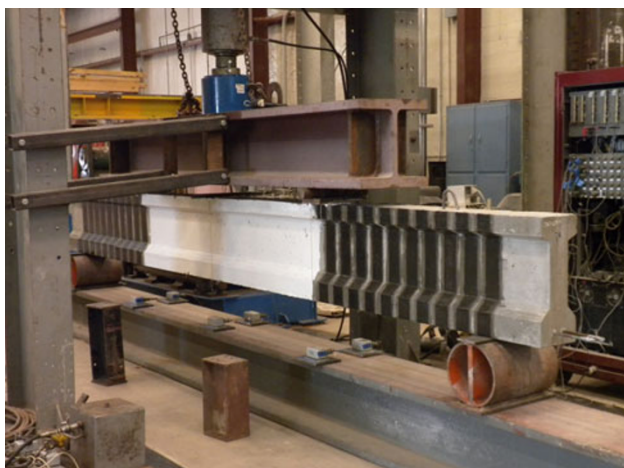
Fig. 6 Transverse straps of FRP placed within shear span (photo by T. Kang).
