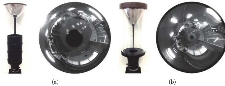
FIGURE 2: Two sample omnidirectional images captured in the same room, from the same position, and using two different catadioptric systems.
