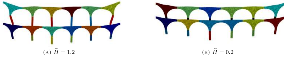
FIGURE 13. Displacement field of the bridge for different values of the height \tilde{H} of (all) the pillars in the third layer; the displacement field is scaled by a factor of 40000.
