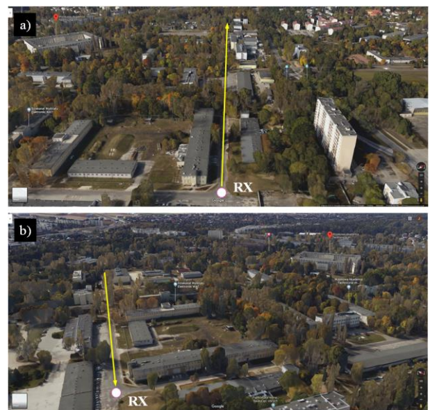
Fig. 12. Spatial placement of initial (a) and final (b) sections of measuring route where LOS conditions occur.
