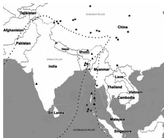
Figure 1. Map of the geographical positions of all of the 10 earthquakes for which the precursor variations were observed (triangles) along with location of the VEF instrument (open circle). The remaining 22 of the 32 earthquakes, where precursors were not observed, are also shown (rectangles). Dashed lines demonstrate the limit of Eurasian, Indian and Australian plates.
