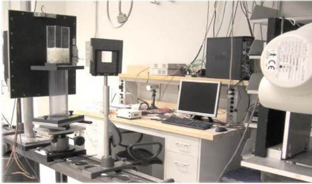
FIG. 4. Experimental setup for imaging the phantom. To produce angular projections, the phantom was rotated, and the detector and the source were fixed.
