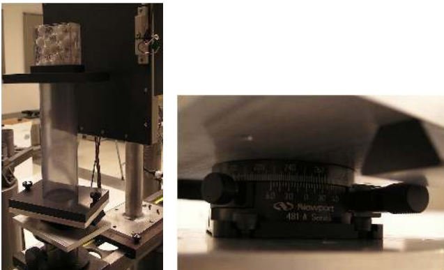
FIG. 5. On the left, the phantom rotator for producing angular projections and its closeup view on the right.
