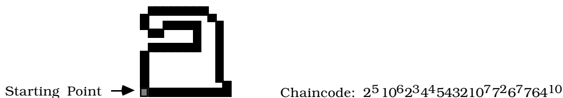
Figure 13: Chain Code of the character “a”. The exponents denote the number of pixels along a certain direction.
