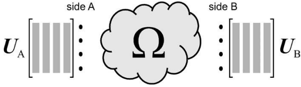
Fig. 1. Parameters required for the new model. The spatial eigenbasis \mathbf{U}_A at side A, the spatial eigenbasis \mathbf{U}_B at side B, and the coupling matrix \mathbf{\Omega} .
