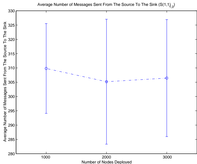
Fig. 37. The number of messages sent as the number of nodes deployed increases.
