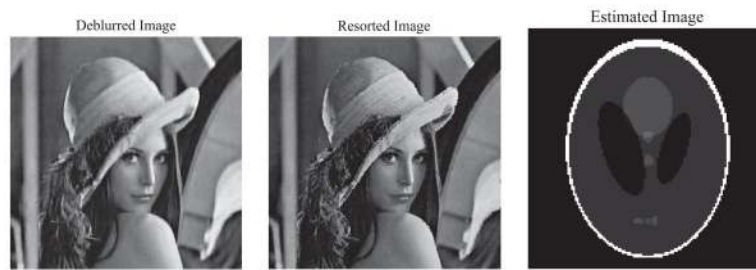
Fig. 12. The deblurred and reconstructed images of Lena, and the reconstructed Shepp–Logan phantom image by strictly contractive PRSM. The SNRs for the reconstructed images are 46.6dB, 57.5dB, and 47.6dB, respectively.
