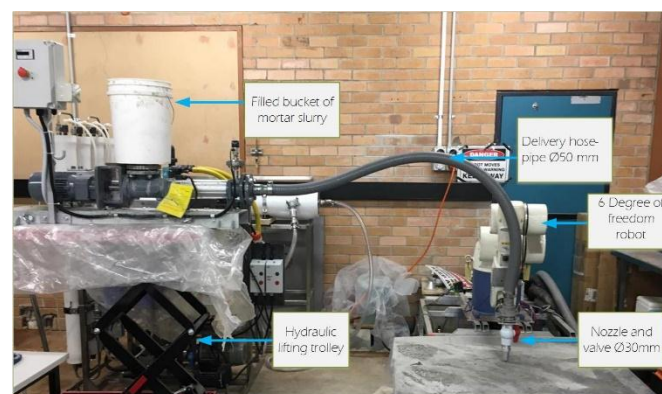
Figure 4. The final system with the progress cavity pump connected to the robot.
