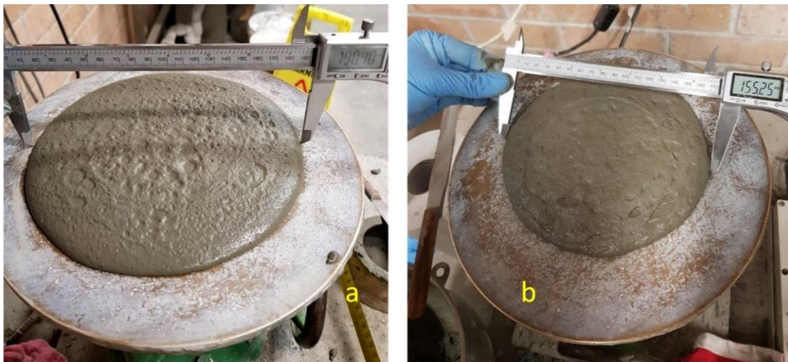
Figure 15. Spread-flow test: (a) For trial 5 which did not use fibre; (b) for the same trial by adding fibre with 1% polypropylene fibre.
