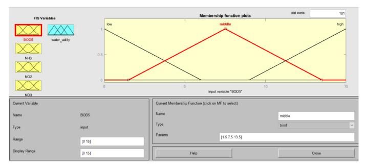
Figure 4. An example of a triangular membership function (BOD<sub>5</sub> indicator).
