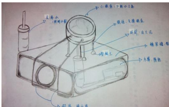
Figure 1. The Design Drawing for the Drainage Mechanism Made of the Iron Drug Box
