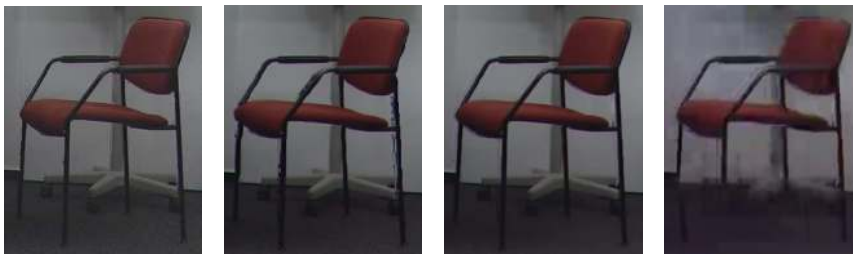
(i) Synthesis from original data, PSNR = 40.1dB (j) PSNR = 36.96dB; Depth = 6% of bit-rate;(0.21bpp in total) (k) PSNR = 39.38dB; Depth = 38% of bit-rate;(0.21bpp in total) (l) PSNR = 34.17dB; Depth = 88% of bit-rate;(0.09bpp in total)
