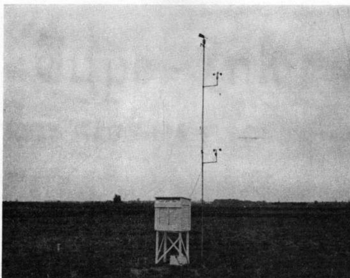
Figure 3. Weather station (instrument shelter and wind system).
