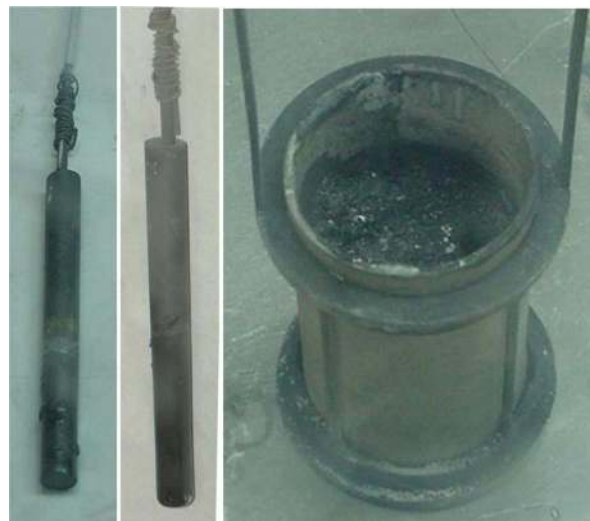
Figure 7. Photographs of the used graphite anodes and the salt. Thick layer of carbon deposit is visible on the top of the salt, contained in the alumina crucible.
