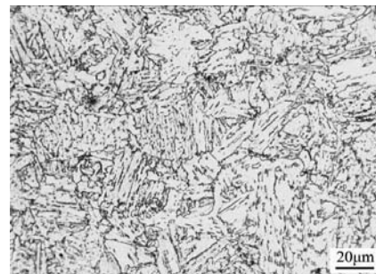
(a) Ordinary X80 pipeline steel
