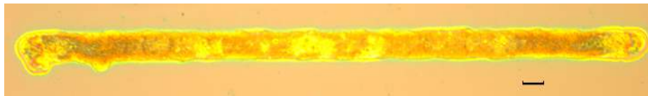
Figure 3.19. A sintered 15-layer line with dot spacing 40\ \mu\text{m} using optimized 5-pass printing at the jetting frequency of 800 Hz. The line was obtained by sintering the printed line shown in Figure 3.18 at 250\ ^\circ\text{C} on the hot plate for 1 hour.
