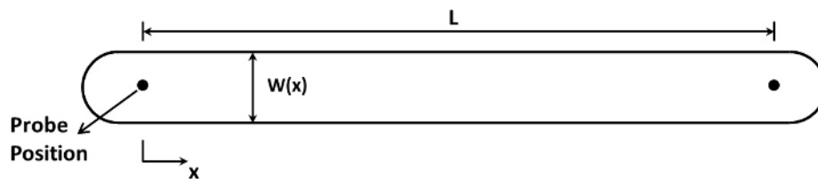
Figure 3.20. Illustration of a general line resistance measurement using 2-probe method.
