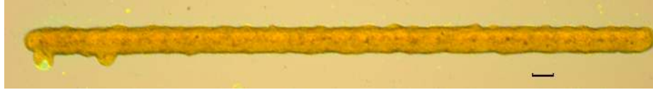
Figure 3.18. A 15-layer line with dot spacing 40\ \mu\text{m} using optimized 5-pass printing at a jetting frequency of 800 Hz. The calibration bar represents 100\ \mu\text{m} .
