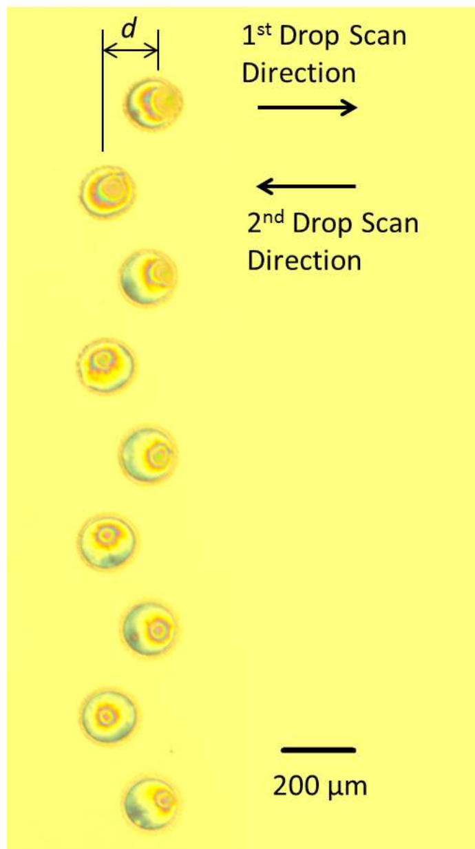
Figure A.1. Equidistant dots in a vertical line were printed bidirectionally with a drop pitch 250 \mu\text{m} and a stage scanning speed 225 \text{ mm/s} . The scan direction was defined as the relative motion of the print head with respect to the substrate.
