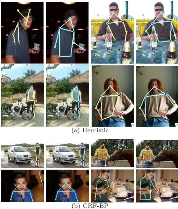
Fig. 15 Comparison of the tree graphs to their respective fully connected models. Left images are inferred results using the tree, right images using the complete graphs. If parts are missing the tree-graphs get disconnected and independent subgraphs are matched, leading e.g. to spurious legs inside the body: (a) 1st row, (b) all except first pair. Also if a body part is not at its usual location relative to other parts this can cause confusion between symmetric parts (folded arms, (b) 2nd row, right image).
