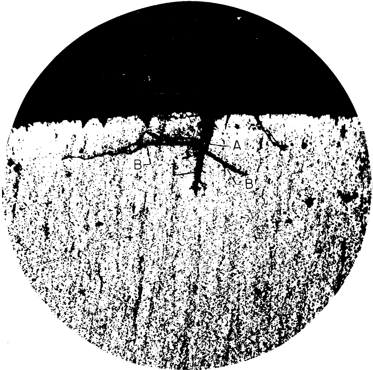
FIGURE 9.—Typical early failure stage in polar area. SAE 52100; X100.
