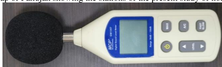
Figure 2- Auto range RS-232 sound measuring device used in the present study.
