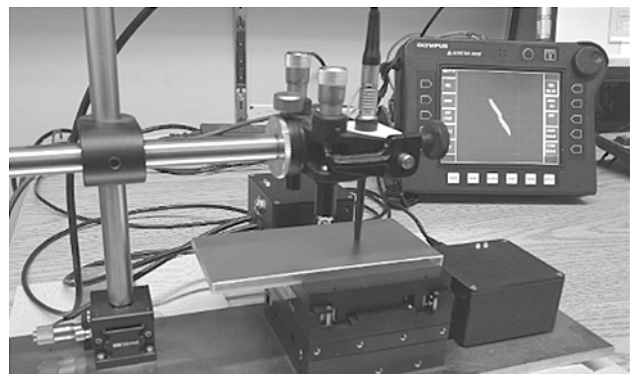
Fig. 1 Experimental setup for performing automated ECT scans
