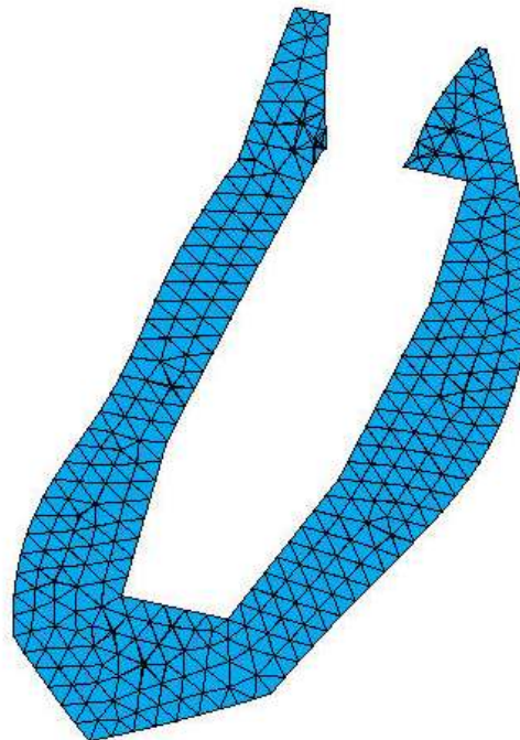
Figure 2. Cross section view of fracture depicting triangular contact elements.
