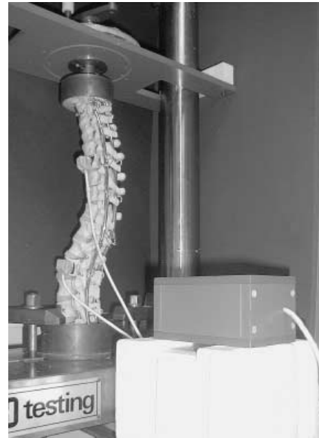
Fig. 4 Sensors of the Fastrak equipment are attached to the T6 and T12 vertebrae. The transmitter placed in front of the construct emits low-frequency magnetic field signals. The sensors pick up the field signals and transmit them in digital format to the computer, allowing it to calculate the movement produced within the construct in six degrees of freedom
