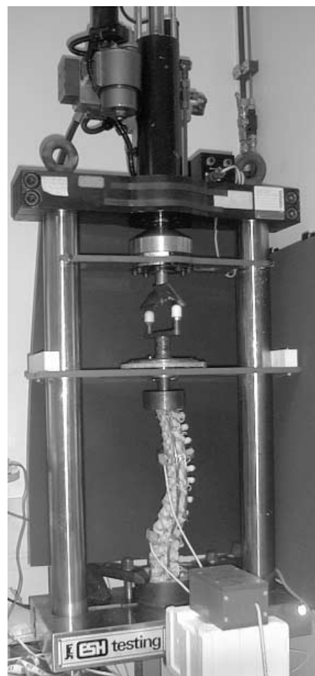
Fig. 2 The construct has been mounted for testing on the electro-servo-hydraulic machine. The Fastrak sensors are secured to the T6 and T12 vertebrae. The transmitter that emits magnetic field signals is placed in front of the assembly
