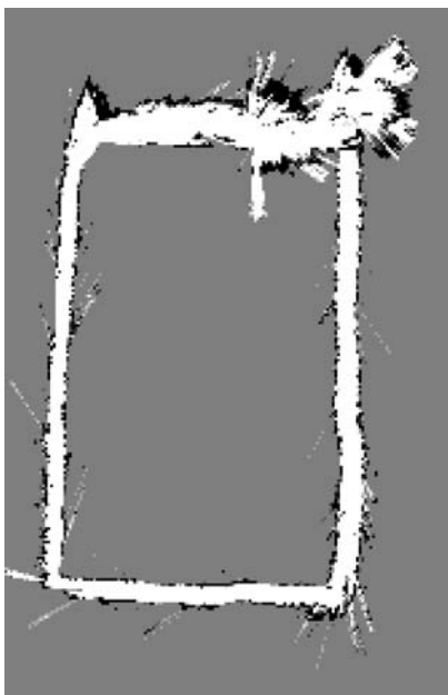
Figure 11. The occupancy grid constructed using the camera location for the maximum likelihood trajectory in Fig. 10. In the grid, white pixels represent empty space while black pixels represent occupied space. Gray pixels denote unobserved areas. The grid’s resolution is 15 \times 15 cm.
