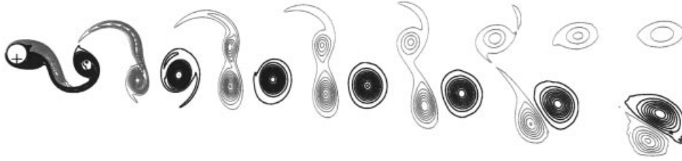
FIGURE 14. Vorticity contours for the oscillating cylinder on the A_2 solution branch (figure 8) for the asymmetric synchronized mode, F = 0.904 .
