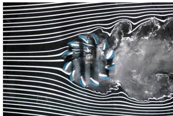
(a) Shutter speed 1/4000 s (momentary streamlines).
