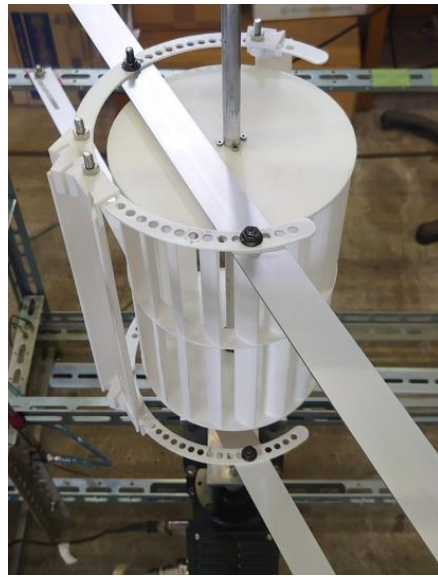
Figure 6. Setting appearance of a cross-flow wind turbine test model with three flow deflectors.
