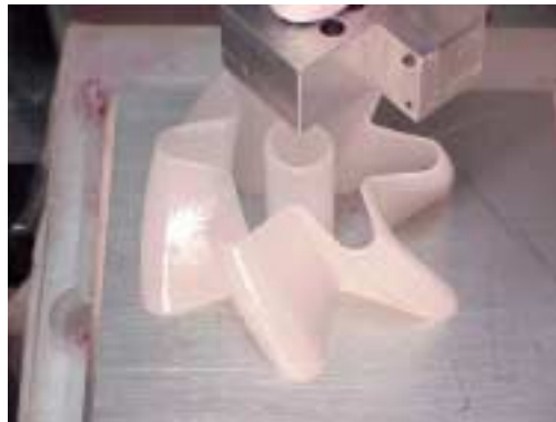
Figure 2: An ice part built by RFP
