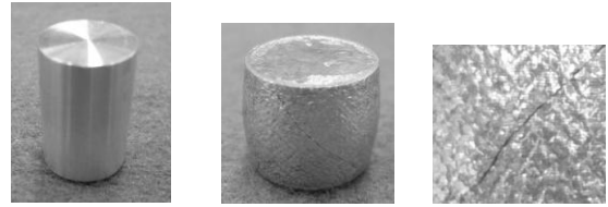
Fig. 1 Compression test of Al-Zn-Mg-Sc Alloy before heat treatment
