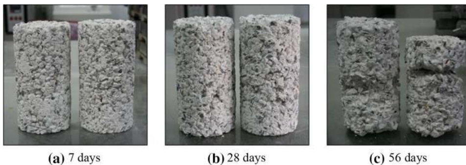
Fig. 16 Images of cementless binder porous concrete after immersion in 5 % H 2 SO 4 .
