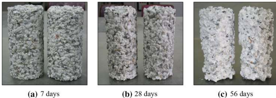
Fig. 15 Images of OPC porous concrete after immersion in 5 % H 2 SO 4 .
