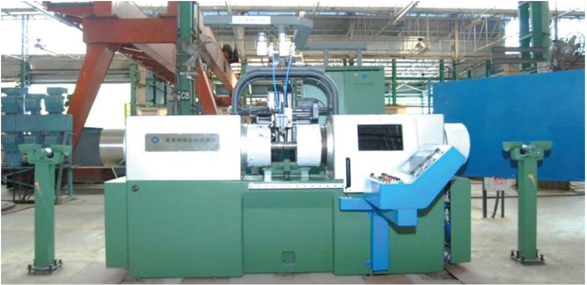
Figure 2: Photograph of HW-GTAW setup.
