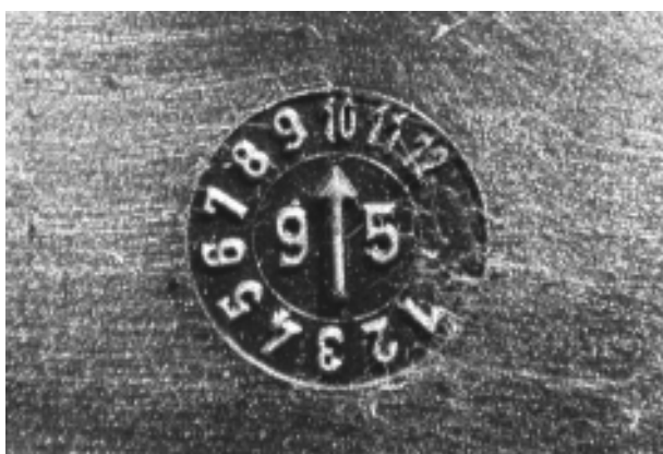
Fig. 8 The date clock on grips panel of Sig Sauer pistol indicates October 1995
