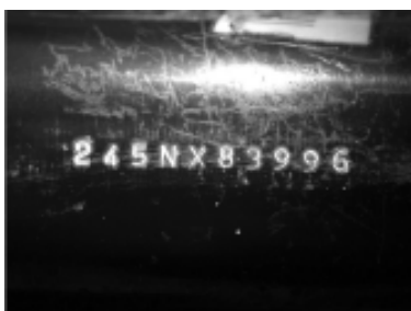
Fig. 1 The "NX" in serial number of Browning pistol indicates the year of 1993
