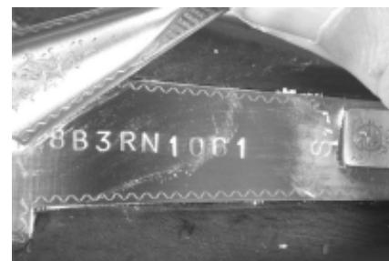
Fig.2 The "RN" in serial number of Browning shot-gun indicates the year of 1979
