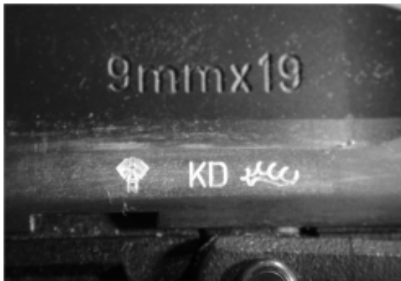
Fig. 6 The "KD" proof marks on the slide of HK pistol indicate the year of 1993
