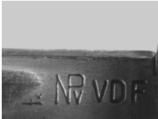
Fig.3 The "VDF" in proof marks of Glock pistol indicates November 1994
