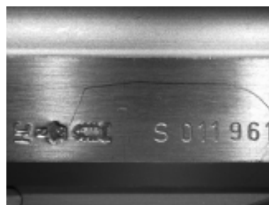
Fig.5 The "JH" proof marks on the slide of Sig Sauer pistol indicate the year of 1987
