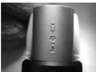
Fig.4 The "JE" proof marks on the frame of Sig Sauer pistol indicate the year of 1984
