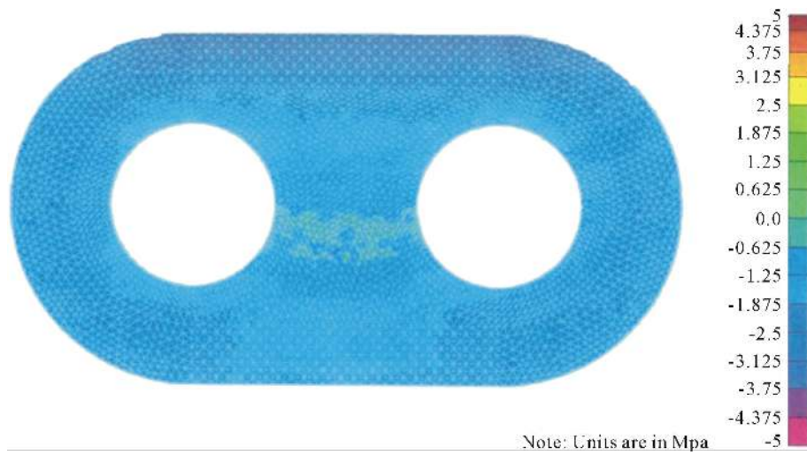
Figure 25. Major Principal stress contour for solid element model.
