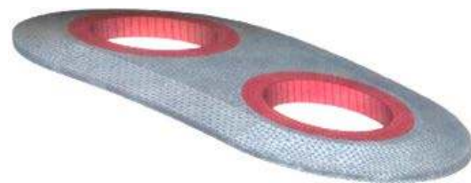
Figure 6. Isometric view of solid element model showing embedded steel plates around SG openings.
