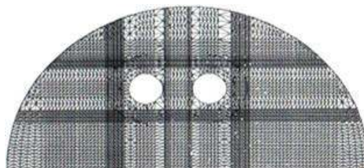
Figure 8. Plan view of mesh type-2 for layered shell analysis.
