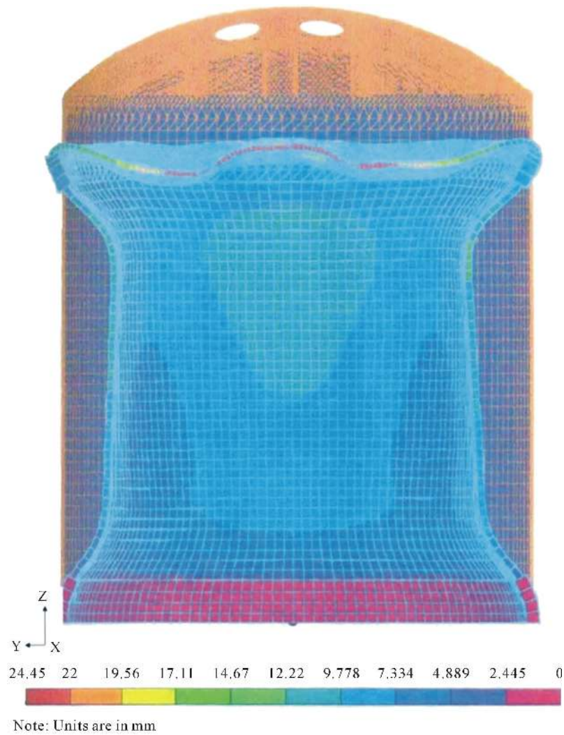
Figure 12. Total displacement contour with deformed shape for the layered shell model in elevation.
