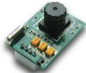
Fig 6: A camera-based wireless sensor device
