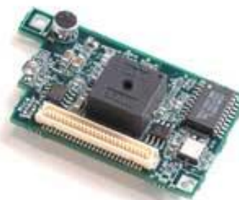
Fig 7: Acoustic wireless sensor device
