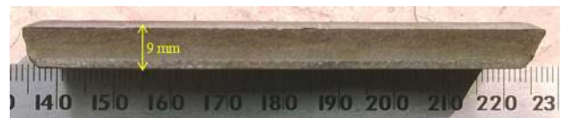
Fig. 19 Defect-free hot worked plate obtained from slab sample without intercolumnar crack
