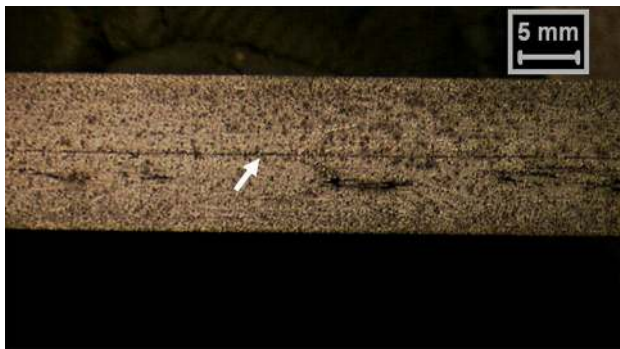
Fig. 1 Crack-like defect at centerline of hot-rolled product arising due to centerline segregation
