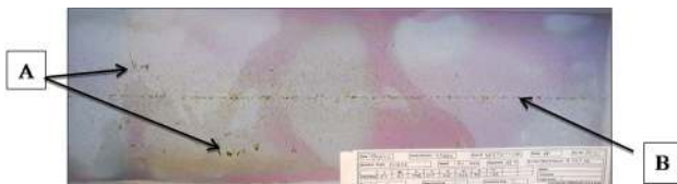
Fig. 6 Sulfur print plate of transverse section of a cast slab showing (A) intercolumnar cracks and (B) centerline segregation
