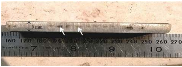
Fig. 15 Defects in hot worked plate sample arising from intercolumnar cracks in the slab sample
