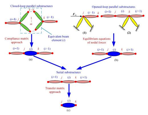
**Figure 4.** Illustration of serial and parallel substructures: (**a**) the closed-loop parallel substructure; (**b**) the opened-loop parallel substructure; (**c**) the series substructure.
