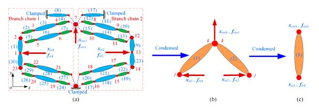
**Figure 9.** Condensed topology of the compliant amplifier: (**a**) numbering and discretization; (**b**) the equivalent topology; (**c**) the equivalent beam element.
