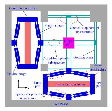
Figure 8. The 2-DOF precision positioning platform.
