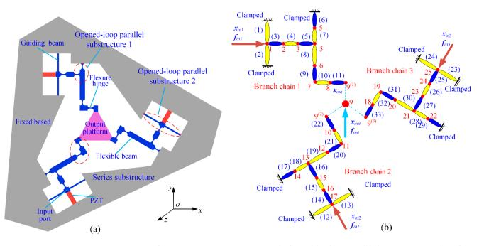
Figure 13. The 3-DOF precision positioning platform: (a) schematic; (b) discretization and numbering.
