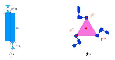
Figure 6. Nodal displacements and nodal forces: (a) the flexible beam; (b) the lumped mass.
