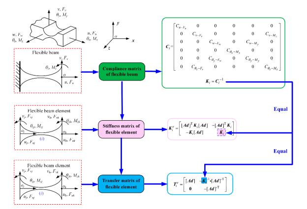
Figure 2. Transfer matrix of a flexible beam element.
