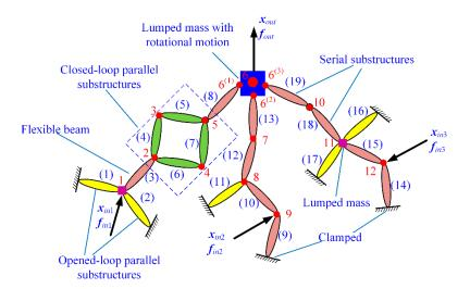
Figure 5. General topology of typical compliant mechanisms.
