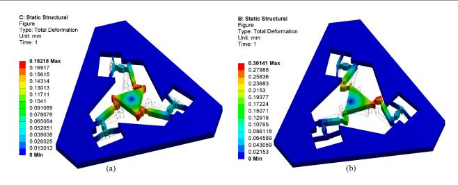
**Figure 15.** Finite element results. (a)  $f_{in1} = f_{in2} = f_{in3} = 100$  N; (b)  $f_{out} = [0 \text{ N}, 50 \text{ N}, 0 \text{ N}, 0 \text{ N} \cdot \text{m}, 0 \text{ N} \cdot \text{m}, 1 \text{ N} \cdot \text{m}]$ .
