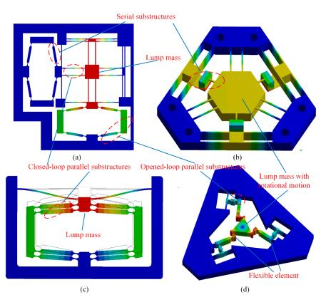
**Figure 3.** Typical compliant mechanisms: (**a**) a *XY* monolithic precision platform [35]; (**b**) a monolithic tip-tilt-piston spatial compliant manipulator [35]; (**c**) a one-dimensional precision positioning platform [38]; (**d**) a 3-DOF precision positioning platform [24,35].
