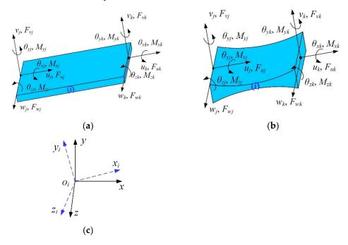
Figure 1. Nodal displacements and nodal forces of flexible elements: (a) the flexible beam with equal-section; (b) the flexible beam with variable-section; (c) the local and reference coordinate systems.
