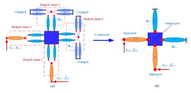
**Figure 10.** The 2-DOF precision positioning platform: (**a**) numbering and discretization; (**b**) the equivalent topology.
