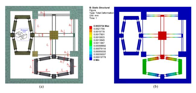
Figure 11. Finite element analysis. (a) geometric parameters; (b) result of one simulation set.
