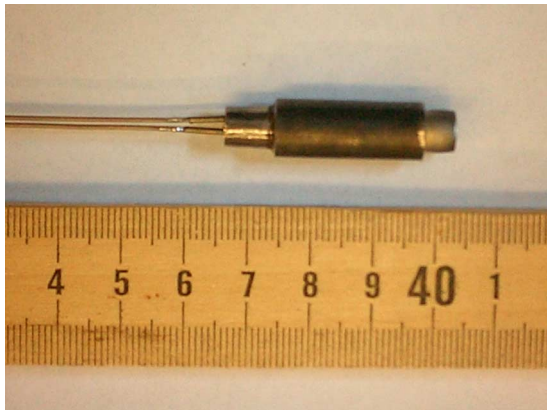
Fig. 3. Photograph of a splice assembly to join two multifilament \text{MgB}_2 wire inside Cu alloy matrix.
