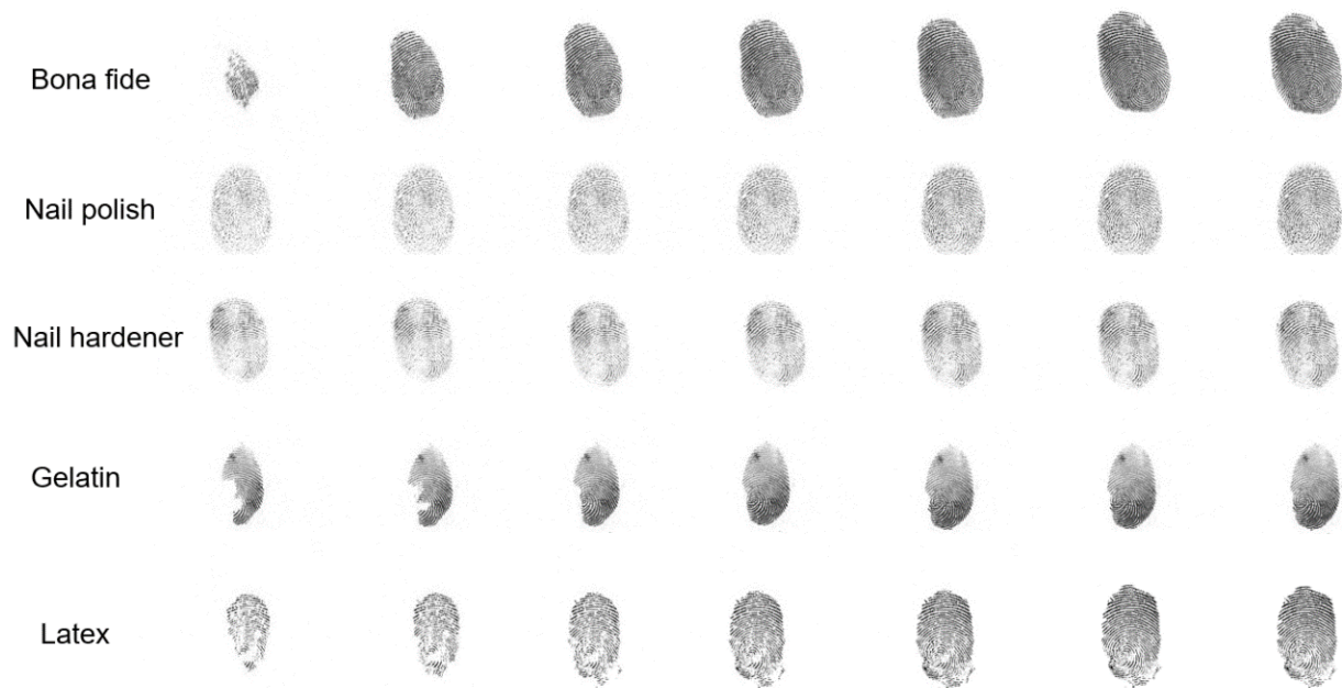
Figure 4.4. Optical sensor captures. For reasons of space, this figure shows partial examples of bona fide and attack presentations (The average number of frames/presentation is 25).
