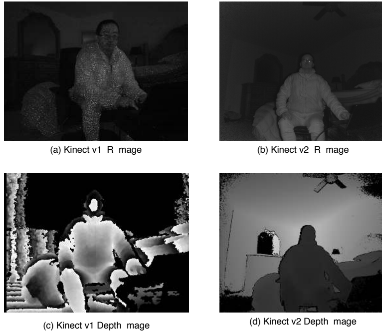
Fig. 4. Comparison of the IR and depth image quality between Kinect v1 and Kinect v2. The two sets of images were taken with the maximum resolutions and with the same Kinect-to-user distance. As can be seen, not only the quality of Kinect v2 images is obviously higher, the field of view is wider as well.
