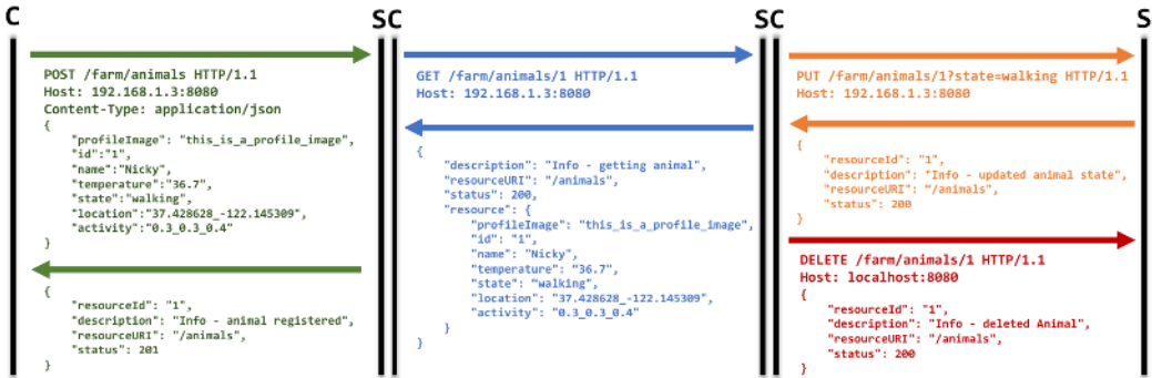
Fig. 8. Example of REST HTTP methods for CRUD operations; C: Client, S: Server)
