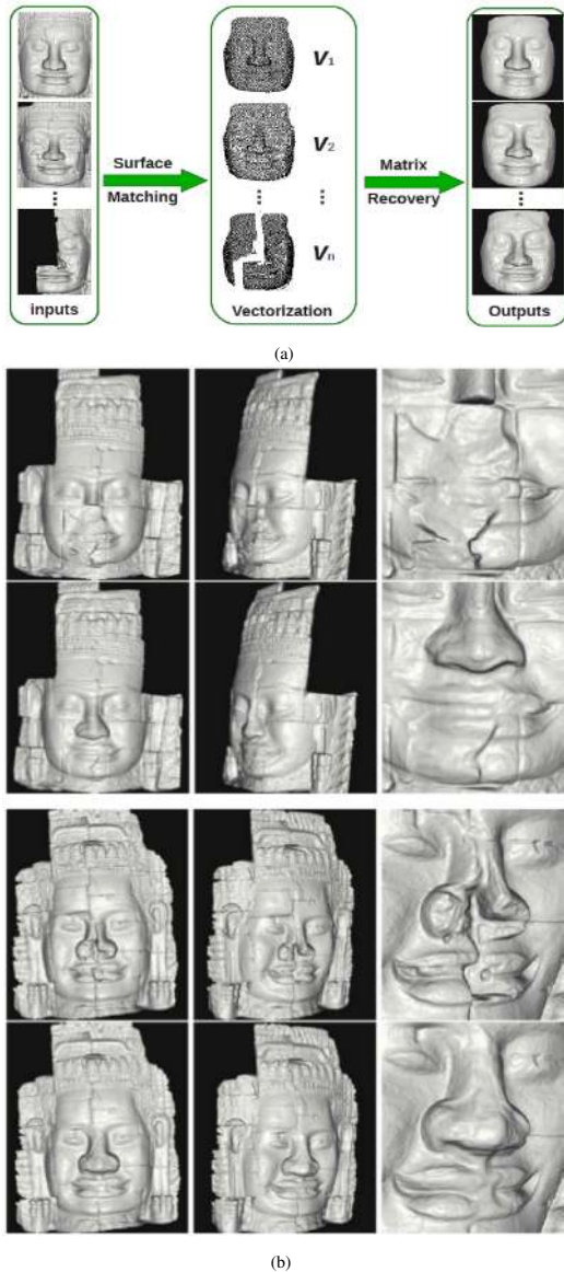
Figure 27: Restoration of statues from many-to-many analysis. (a) the basic idea behind restoration of collection of object. After aligning of all 3D models, dense correspondences are found. A vector representation of each input shape is computed from the correspondence sets, and matrix recovery is applied to restore missing parts; (b) examples of restored results (upper model is the measured shape, while the bottom one is the restored output). Courtesy of Lu et al. [LZT*11].
