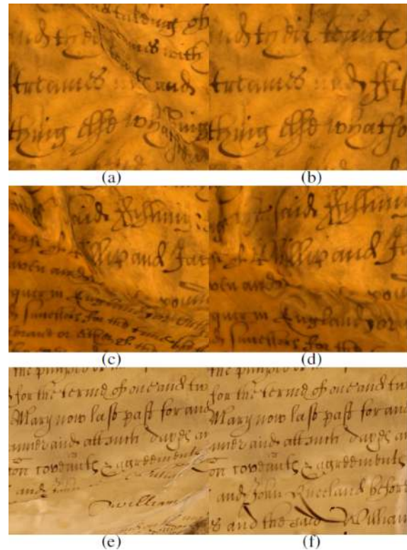
Figure 13: Interactive browsing of damaged documents. Severely damaged documents are acquired in 3D using a Structure-from-Motion approach. A dynamic flattening is performed while the user browses the document in order to increase its readability. We show sections of the mesh rendered in local-affine mode without flattening (left) and with local-flattening mode (right). Note that the original wrinkles remain visible since the shading is baked into the texture [PTW13b].
