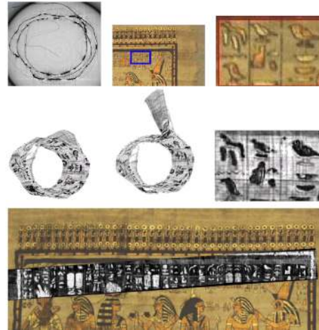
Figure 22: Volumetric scanning of a rolled papyrus. Top: one slice of a CT-scan, a digital image of the original item, and a close-up view. Center: two views of the particle system simulation, and a detailed view after unrolling. Bottom: a comparative evaluation by overlapping the unrolled information from CT-scan and the original papyrus. Courtesy of Seales et al. [SL04].
