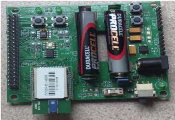
Figure 8: Jennic active RFID Tag (Ref. 29)
