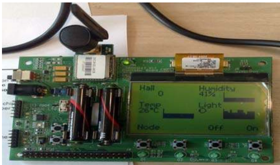
Figure 9 : Jennic active RFID reader (Ref. 29)
