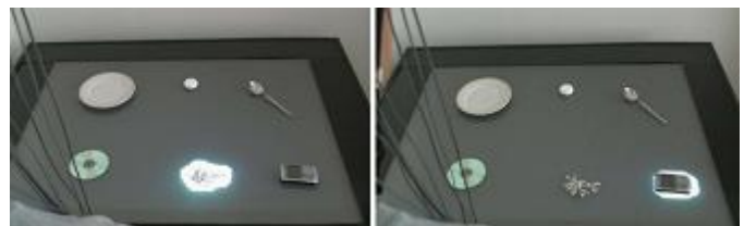
Fig. 6. Multitouch display interface, where objects are enlightened one by one, triggering a P300 wave. Source: [37].
