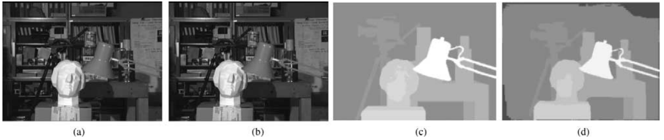
Fig. 4. Matching result from the graph cut algorithm [40]: (a) left image, (b) right image, (c) ground truth disparity, and (d) computed disparity.
