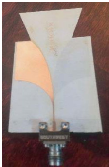
(a) Fabricated AVA with metamaterial
