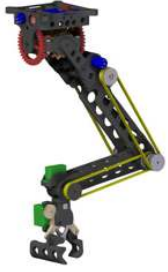
(a) Arm with motors close to base, and motion transmission with belts [15]
