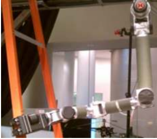
(e) A dexterous manipulator on a UAV simulator [50]
